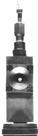
Fig. 1. The hydrostatic pressure cell viewed from the exit-window side; constructed of brass with a length of PEEK tubing (SIGMA, HPLC equipment) transmitting the pressure.
